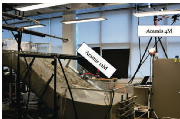
Figure 2 Setup of the optical measuring system in models subjected to static loading conditions (simulated rainfall).
